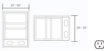
The window installation kit allows you to install the air conditioner in most vertical sliding windows 25" to 50" wide, or horizontal-sliding windows from 18" to 50" high.
