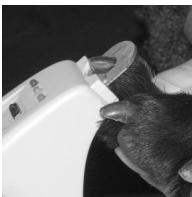
*The lights will change from RED to GREEN as the sensor moves outward from the base of the nail to the tip where the quick is no longer present.*
