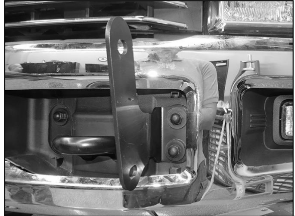
(Fig 4) Reuse factory bumper bolts to attach driver/left Frame Bracket to bumper
