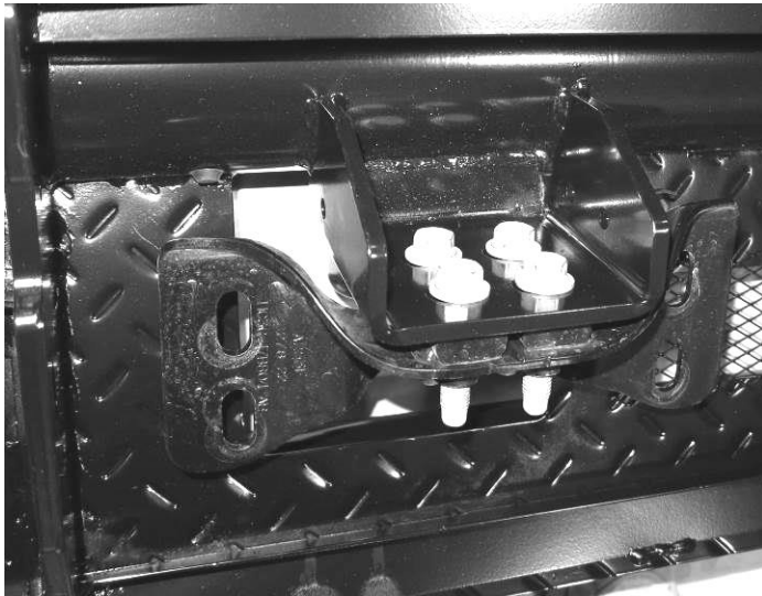
(Fig 7) Reuse factory hardware to attach tow hook to mount on back of HD bumper
