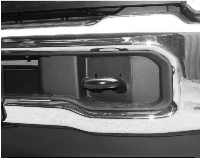
(Fig 3) Remove plastic cover around tow hook
