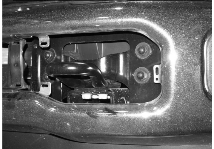
(Fig 4) Remove bumper bolts (driver side pictured)
