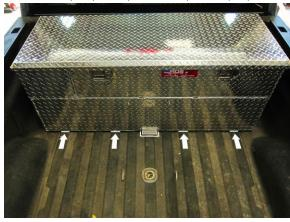
3) Drill one 5/16" hole in each tab and the bed of the truck (making sure as to not hit any wiring or other critical components of the truck) for mounting. Drill only one hole per tab. Place a bolt in your first hole to help keep the tank in-place while drilling the other holes.
