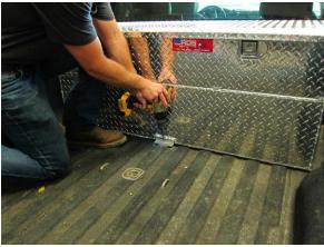
4) Mark a spot in the side bed that best aligns with the drain plug. Now move the tank out of the way and drill a ¾" hole in the bed for the fuel hose.
