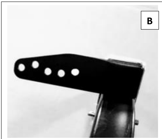
Crossbar setting for rear leaning ROPS.
