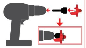
3. Screw the horizontal nipple into the container using the drill and the installation helper. Make sure the gasket is positioned at the end of the threads before installing. Do not over-tighten horizontal nipple using the drill bit.
