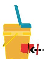
Hold the port upright and 7 twist the locknut onto the threads, turning until tight.
