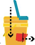
\* The gasket belongs on the inside of the container. The gasket should be in-between the both the port and the container wall.
