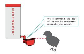
1. Hold the **DRINKER** on the outside of the cage and screw the cup into the drinker from the inside.
