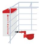
2. Secure the drinker to the cage-wire using the SPRING CLIP.
