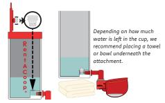
2. Unscrew the drinking attachment by its elbow.
