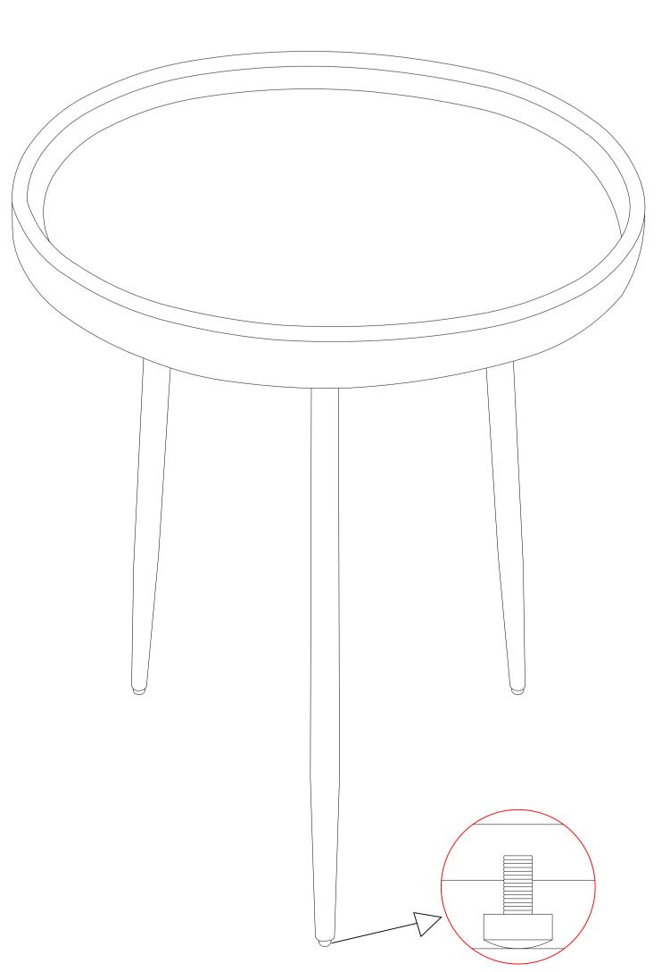
Note: Levellers are provided at bottom to balance the product on uneven surface.
