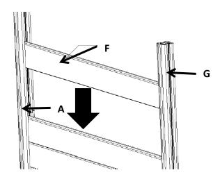
5. Insert the side bar, fitting the top cover to the post, and fasten with a corner clip.
