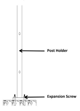
2. Drill the **Square Bottom Post** into the existing concrete with four expansion screws. The distance between centers of two posts is 72". Insert the post inside the post holder.
