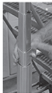
When lowered the pole sections should not go all the way inside the lower pole section(s).
