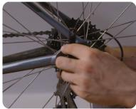
**3.** If your bike's wheel uses a bolt through axle i.e. with a nut at both end of the axle, there is no need to use the provided replacement skewer because a skewer doesn't work with wheels that have a bolt through axle. However, the couplings will need to hold the frame firmly to ensure no movement.
