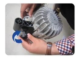
**3.** Attach the adjustment knob with clockwise motion, but do not over-tighten.
