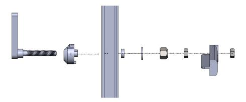
**Step 5:** Slide the Spacer then the washer onto the threaded stud.
