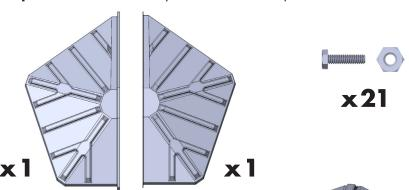
Step 2: Bolt the two roof panels together using 1" bolts through pre-drilled holes
