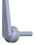
Step 4: From outside the blind, slide the threaded stud of the handle through the pre-drilled hole with the handle in a vertical position; the collar should sit in the large and small pre-drilled holes
