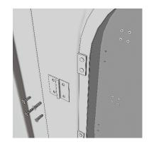
**DO NOT** over tighten hinges to the plexiglass; this can cause the window to crack. Tighten nuts by hand or with a socket **DO NOT** use Loctite
