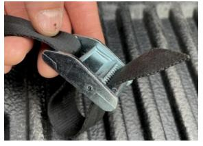
Step 3: Adjust clasp and cover toward cab approximately 65". Repeat on the passenger-side.
