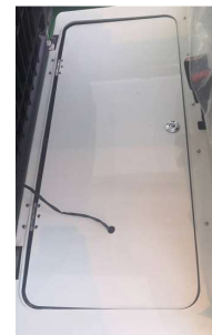
Battery Compartment Isolator plate
