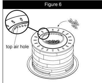
7. After the fire pit has cooled down completely, take out the chamber and empty the ash, cover the fire pit with the outdoor weather cover when not in use to protect it from the elements or when fire pit is cool COMPLETELY after the use.
