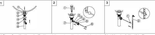
1-1. Remove flange (1), rubber washer (2), rubber washer (3), steel washer (4) and mounting nut (5) from the pop-up assembly.
