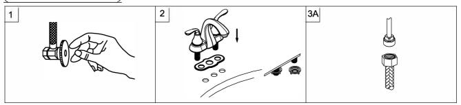
1Shut off water supplies. Remove old faucet. Clean sink surface in preparation for new faucet.
