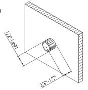
Place Mounting bracket (16) onto pot filler(1) Mount pot filler onto nipple on the finished wall surface, do not full tighten the body to the wall and mark three mounting holes. Ensure that mounting holes will be clear of all concealed pipe work.
