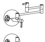
The nipple must be sealed to the wall to prevent water entering the wall cavity. Apply thread tape to nipple. Place the washer(18) and screw wall mount bracket(16) to the wall.
