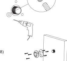
Note: The mounting bracket must be fully attached to the finish wall.
