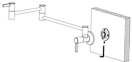
After installation, remove the aerator and turn on the water to remove any debris in the piping. Re-assemble aerator. This tap is equipped with two shut off valves, the wall valve should be closed (handle in vertical position) when faucet is not in use. If the pot filler is to be left unattended, please ensure both valves are left in closed position.
