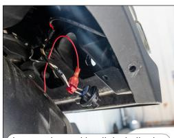
Locate the parking light bulb plug. T-Tap the red wire to the white with brown striped wire for power. Turn on park mode to test.
