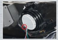
E) Here is an image showing the wires routing through the back of the projector housing. Be sure to route the wires first before installing the halo.
