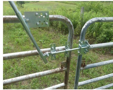
The latch consists of a fulcrum, toggle, sliding bolt, guides, and a receiver. The set is designed so that it can be mounted either right or left. You just need to reverse the bolt on the toggle.
