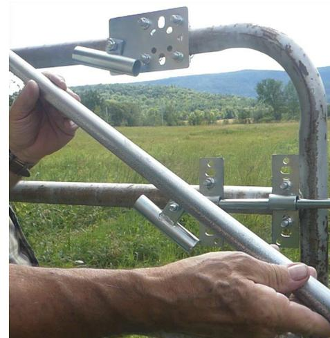
Different gate setups will require different handle lengths therefore, we designed the set so that all you need to do is get some 3/4" EMT conduit – available at any home improvement store – and cut it to the desired length.
