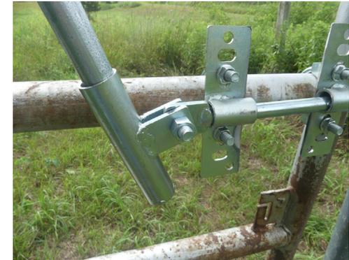
You will want to locate the first guide directly across from the receiver and the second one about 6" back. Then the fulcrum roughly 6" behind that on the next higher tube. For best results use the top horizontal tube on the gate and the next one down. The first cowboy latch you install may require a little adjusting to get things working just right, after that the next will be easy.
