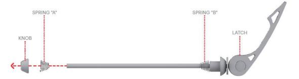
Step 4: Locate the side of the front wheel with the disc. Insert the end of the quick release axle through the hole in the center of the wheel on the side OPPOSITE the disc and push it through to the disc side.
