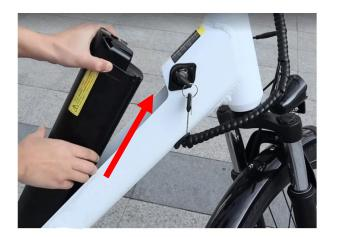
Reinstall battery by sliding the bottom of the battery into the battery compartment and sliding the battery in a downward motion locking it into the battery compartment.
