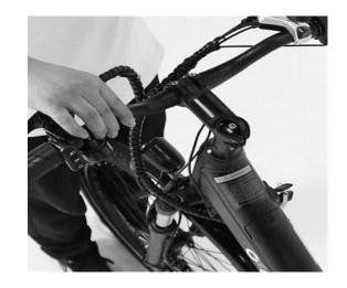
Step 2: Tighten the top screw. When you are finished tightening the screw, add the small rubber cap.
