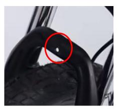
Step 2: Slide front fender through the front fork and over the tire until the tab on the fender meets the fork.
