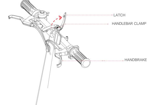
Step 2: Rotate the handlebar forward or backward to reposition it.
