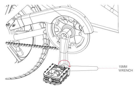
Step 3: Finish inserting and then tightening the spindle into the crank arm by turning it clockwise with the 15 mm wrench or 15mm wrench tip of the multi-tool.
