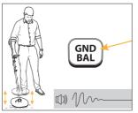
Ground Balance (if needed to eliminate ground response).
