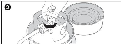
To turn on fuel, turn valve on Gas Growler **COUNTER CLOCK-WISE** to open fuel source.
