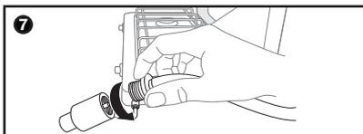
To disconnect device, loosen smaller, metal end of hose from stove, heater or appliance by turning **COUNTER CLOCK-WISE**.
