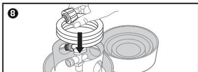
To store, detach hose from tank and coil tightly before placing around fuel valve and zipping the top closed.
