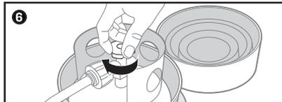
To turn off fuel, turn valve on Gas Growler **CLOCK-WISE** to close fuel source.
