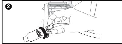
Use smaller, metal end of hose to connect to stove, heater or appliance by turning **CLOCK-WISE** to tighten.
