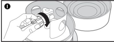
To connect Gas Growler, fasten black collar end of hose to tank valve by turning **CLOCK-WISE** to tighten.
