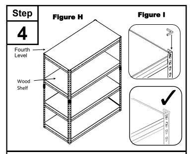
Add a wood shelf to the previously built level, then continue by adding the fourth level to the unit using two (2) beams and two (2) braces per level. Tap lightly to properly seat the rivets and add the final wood shelves to the unit (see figure H). Finally place the four (4) post caps on the top of each post (see figure I). Double check to make sure all rivets are fully engaged into the narrow end of the post slots. Assembly is now complete.
