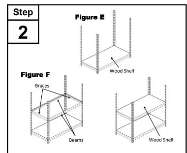
Add a wood shelf to the level previously built (see figure E), then continue working by adding the second level using two (2) beams and two (2) braces in the post slots of your desired location (see figure F). Again, place the rivets of the beams and braces into the post slots with the shelf ledge facing up and tap lightly to seat the rivets. Add a wood shelf to the second level.
