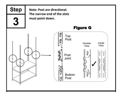
Assemble four (4) posts to the four bottom post assemblies by using four (4) of the post joints. Place the post joint into the top of the bottom post assembly and tap down to properly seat. Next place a post into the top of the post joint and tap down to properly seat (see figure G). Continue by adding the third level using two (2) beams and two (2) braces just above the post joints. Again tap lightly to seat the rivets.
