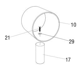
• Assemble the bottom plate(#1)together with all other components(like the picture show on the right) by screw (#21).
