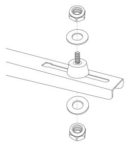
7. Place the air conditioner onto the mounting brackets. Mount the air conditioner onto the brackets using the four (4) dampers. Tighten the dampers to secure the air conditioner.
