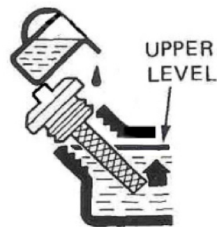
Figure 8B – Adding oil
