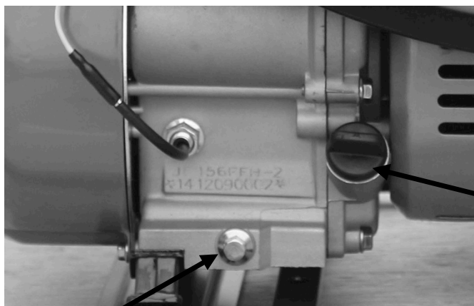
Figure 8A – Use 10mm hex wrench to REMOVE bolt and drain oil
