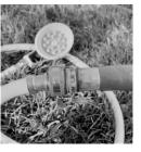
shower brush & water pressure control valve onto smaller end of the white hose.
