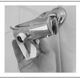
5. Screw original showerhead on front of diverter; tighten with pliers
