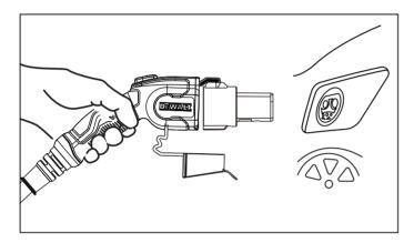
**Step 2:** Firmly plug in the adapter into your electric vehicle.
