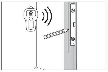
2. Hold the wall bracket against the installation surface. Align the vertical line to the holes of the wall bracket. Firmly mount the wall bracket using the provided screws.
