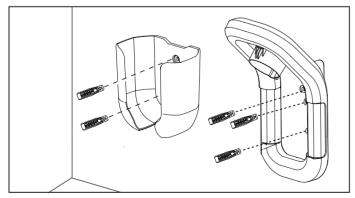
4. Firmly mount the mount holder using the provided screws.
