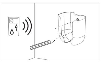
2. Drill the holes into the installation surface.
