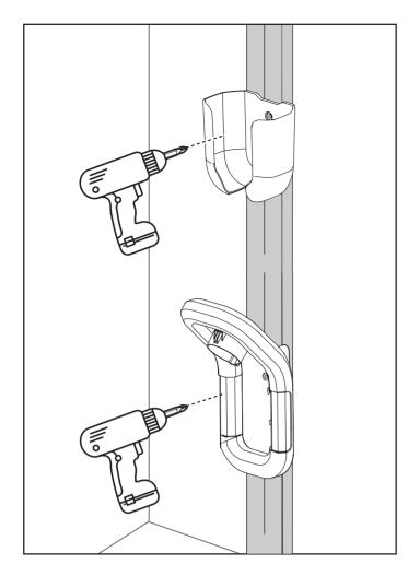
3. Control box inserted into the dock station and charging handle inserted into the charging hook.
