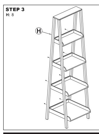
For additional stability, secure the back of the brackets on the back frame to each shelf using two M4x12mm Screws (H).
