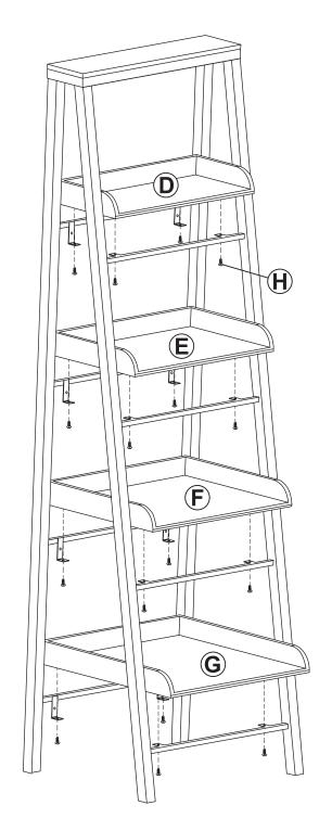
Secure Top Shelf (D), Second Shelf (E), Third Shelf (F), and Bottom Shelf (G) to the bottom of the brackets of the back frame using two M4x12mm Screws (H) for each shelf, as shown.
