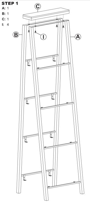
Ensuring the shelf mounting brackets face the center, align Top Panel (C) with Front Frame (A) and Back Frame (B). Loosely secure the top panel my hand-tightening six M6x10mm Bolts (I).
