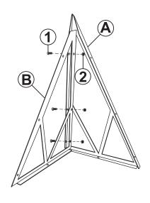
NOTE: Install panels with the mesh screen facing inward.
