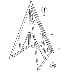
Align remaining Side Panel (B) with the inside of Back Panel (A) and loosely secure by hand-tightening three M6x15mm Bolts (1) and three Nuts (2).
