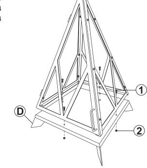
Align the assembled pyramid on top of Base (D) and firmly secure using four M6x15mm Bolts (1) and four Nuts (2).
