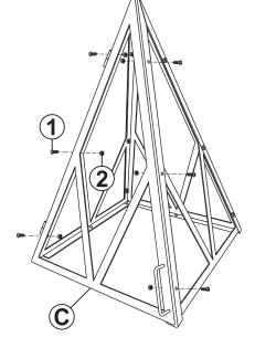
Align Door (C) over the front of the side panels and loosely secure by hand-tightening six M6x15mm Bolts (1) and six Nuts (2).
