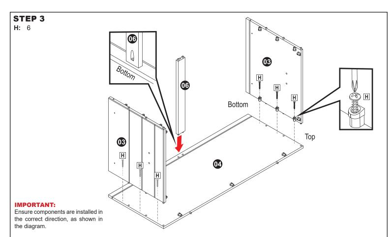
Ensuring the bottom grooves align, secure two Side Panels (03) to Back Panel (04) using six M4.5x25mm Pan Screws (H).
