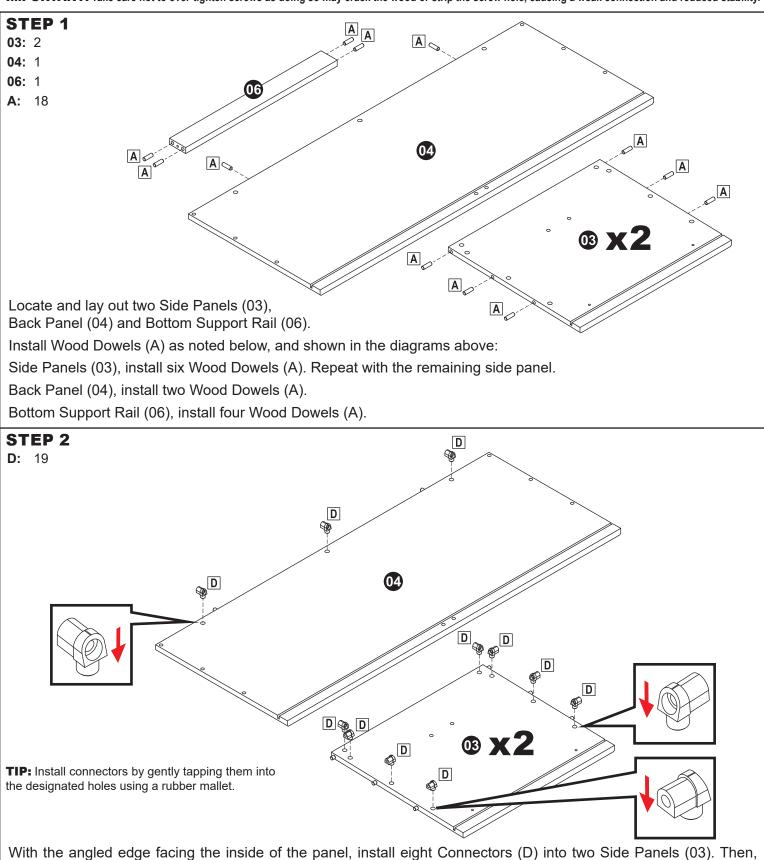
install three Connectors (D) into Back Panel (04).
