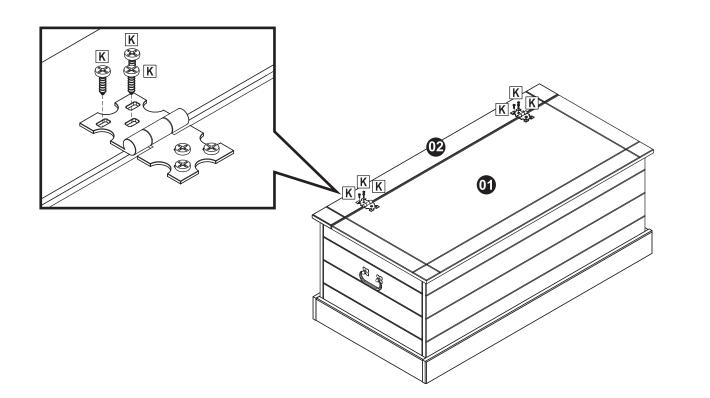
Ensuring Top (01) is aligned with Cap Panel (02), secure the hinges to the cap panel using six M3.5x14mm Pan Screws (K).
