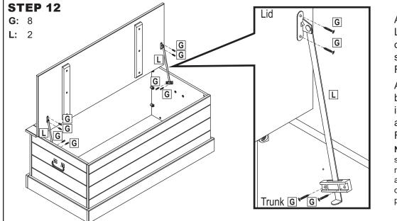
Align the metal mounting plate of Lid Support (L) with the indents on the underside of the lid and secure using two M3x16mm Flat Screws (G).
