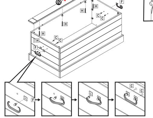
Align the components of Handle Sets (F) with the side panels. Ensuring the handle plates remain straight, secure each handle set using two M4x16mm Bolts (C).
