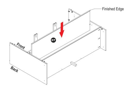
Identify the finished edge of Shelf (07). Slide the shelf into the cabinet, ensuring it is on top of the shelf pins, as shown.
