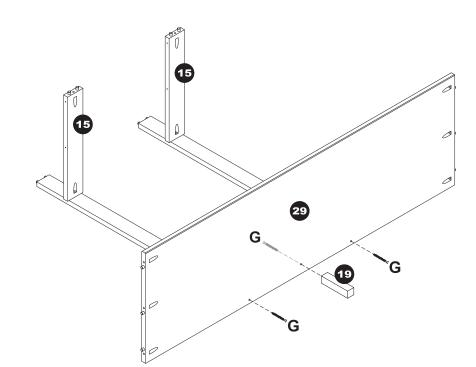
Align the top of Bottom Panel (29) with the back supports, as shown. Secure the bottom panel to each back support using one M4x40mm Flat Screw (G).
