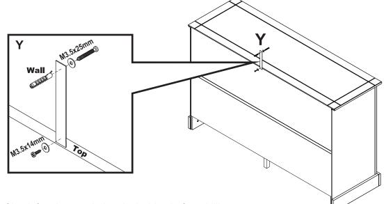
**WARNING:** Check for pipes and electrical wiring before drilling.
