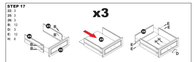
Ensuring the inside grooves align, secure Right Drawer Side (23) and Left Drawer Side (24) to Drawer Face (22) using four M4.5x38mm Pan Screws (B).
