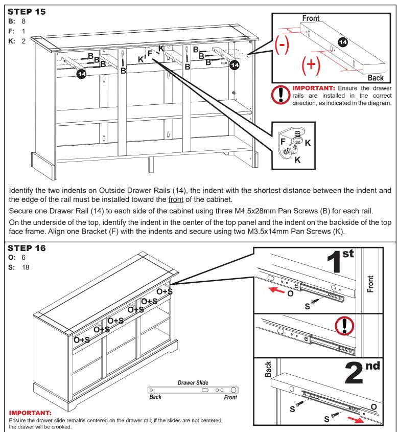
Push the front of Drawer Slide (O) backward. Align the 3rd round hole on the front of the drawer slide with the front indent on the drawer rail and secure using one M4x14mm Flat Screw (S).
