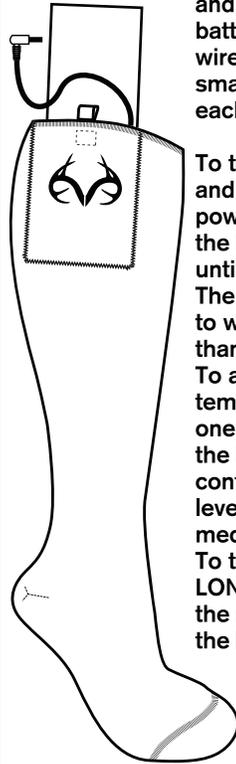
Plug the sock's connectors into each battery pack and place the battery pack and wire inside the small pocket of each sock.
