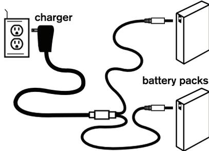
Connect the round power connectors of the charger to each rechargeable battery pack and plug the charger into an outlet. The charge indicator on the charger will turn red while charging; the indicator will turn green when the charge is completed. Disconnect battery packs from the charger.
