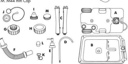
7. Insert water tube through outer hole on sink (B). Next, insert faucet (D) onto water tube that is connected to the base water tank (A). Then, zip tie water tube onto column (C).
