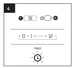
To set the timer power on, while powering off the unit press the Timer button on the control panel (C) or remote control (B).
