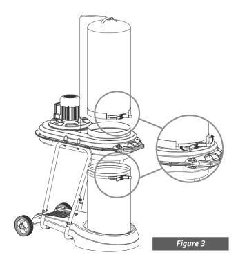
Plug the hose coupling onto the suction inlet on the housing. Secure it in place with the supplied hose clamp.
