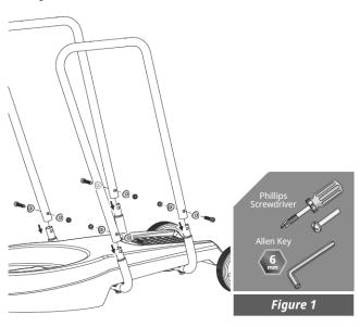
Place the housing assembly on the frame of the pipe supports, align the mounting holes.
