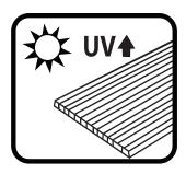
**Note:** The masking film on the polycarbonate sheet indicates which side of the sheet is UV protected.
