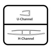
**Note:** Polycarbonate profiles are not intended as a waterproof solution. It is highly recommended that polycarbonate H-channels be installed vertically or with the slope. Installing H-channels horizontally may result in leaking.
