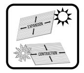
**Note:** Sheets installed in extreme cold or hot weather conditions (even if the holes are pre-drilled) may crack or warp when the temperature fluctuates between the seasons.
