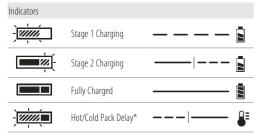
\*The red light will continue to blink, but a yellow indicator light will be illuminated during this operation. Once the battery pack has reached an appropriate temperature, the yellow light will turn off and the charger will resume the charging procedure. The compatible charger(s) will not charge a faulty battery pack. The charger will indicate faulty battery by refusing to light.
