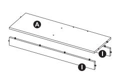
Align Bottom Panel (A) with the dowels in two Toe Boards (I) as
