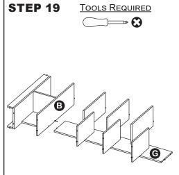
Align the bottom of Top Back Panel (G) with Large Shelf (B) and secure the cam lock.
