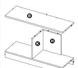
With the spreading bolt facing upward, place Large Shelf (B) onto Divider Panel (K) and Bottom Back Panel (H).
