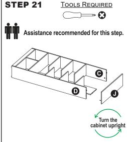
Place Top Panel (J) onto the top of the unit and secure the cam locks. With assistance, lift the unit upright.
