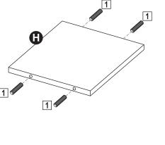
Install four Wood Dowels (1) into Bottom Back Panel (H) as shown.
