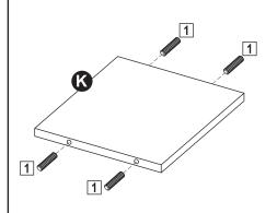
Install four Wood Dowels (1) into Divider Panel (K) as shown.
