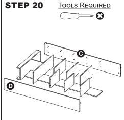
Align Left Panel (C) and Right Panel (D) with the shelves and secure all the cam locks.
