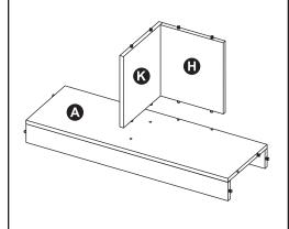
Place Divider Panel (K) and Bottom Back Panel (H) onto Bottom Panel (A) as shown.
