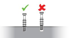
Use a screwdriver to tighten the cam screw until the shoulder is flush with the panel. Do not overtighten or under-tighten.
