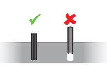
Install wood dowels by gently tapping them into the designated hole using a rubber mallet.
